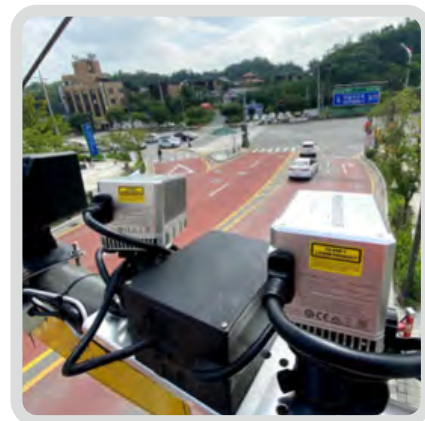
3D sensors monitoring an intersection
