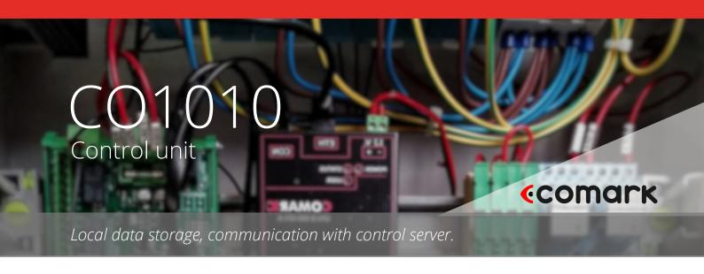
Control unit CO1010 has been designed to be connected to the sensors and to process, archive and send the data received from them.
