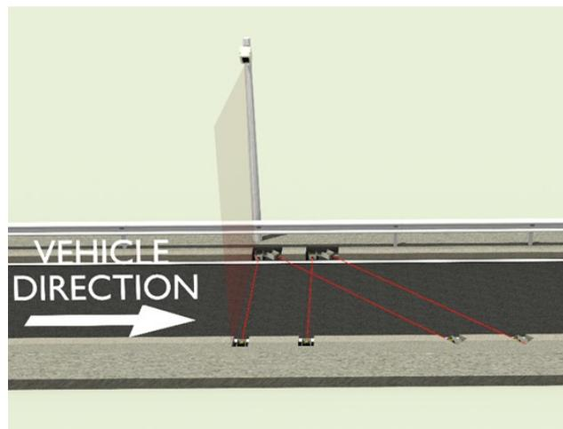
Picture 2: LSR2001-AXLES-4 with 4 photocells
